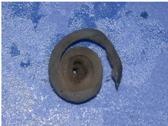
Fig. 13: electroperated cossettes are very flexible and have a high mechanical loading capacity
