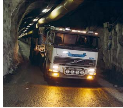
Figure 1. Mine vehicles such as diesel front-loaders and large trucks increase the need for effective ventilation.
