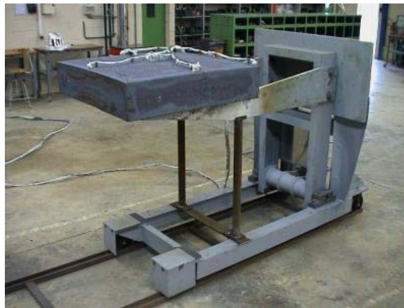
Figure 12 : Instrumented slab on its furnace loader
