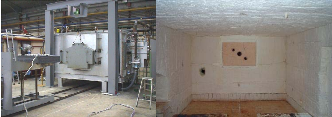
Figure 11 : (a) General view of the test furnace, (b) Internal view of the furnace
