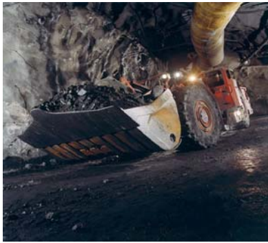
Figure 1. Mine vehicles such as diesel front-loaders and large trucks increase the need for effective ventilation.
