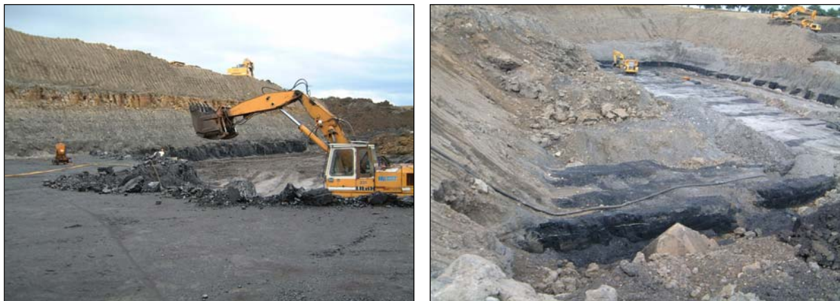
Fig. 2: Opencast coal mining operations: (left) working bench in front of the highwall of a shallow pit. (right) advancing loose-wall (on left) behind working bench
