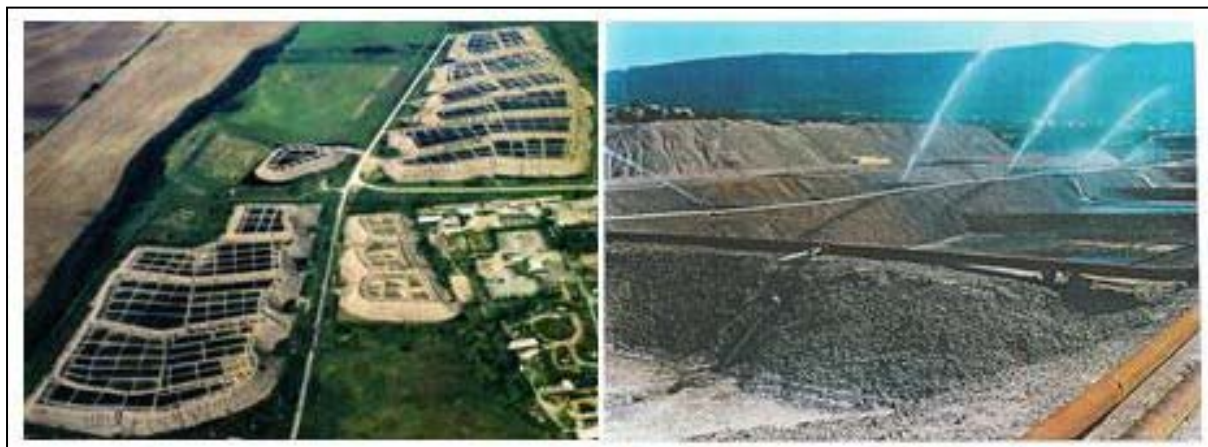
Fig. 3: Alkaline heap leaching at the former uranium mining and processing site near Pécs.
