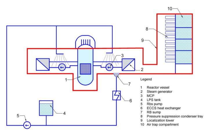
Figure 9- Schematic diagram of VVER-440/213 containment system
