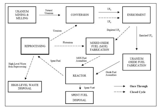
Figure 13 - Open and closed fuel cycle
