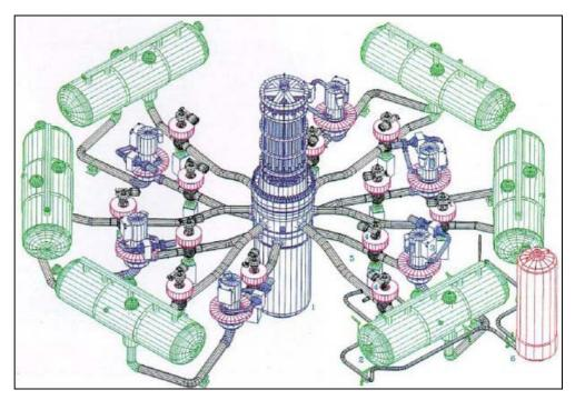
Figure 7 - Primary circuit representation with the six coolant loops
