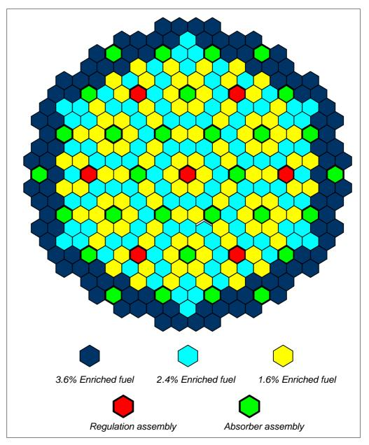
Figure 11 - Layout of the first core for MO34
