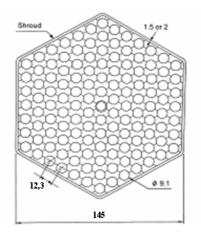
Each fuel assembly is covered by a shroud, as shown in Figure 12.
