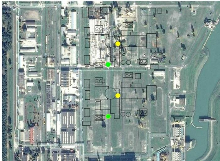
Figure 20.6.2-1: DBC4 event emission points (green: chimney; yellow: building fan).
