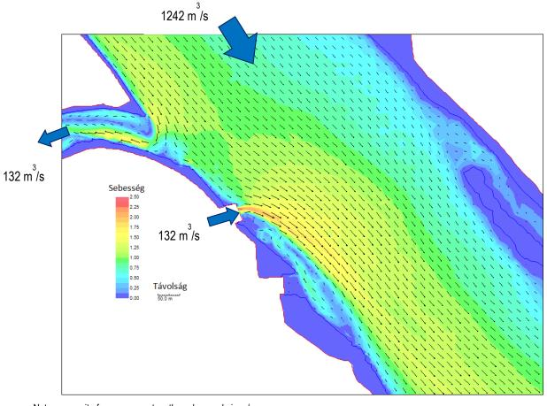
Note: unit of measurement on the colour code is m/s Legend: Sebesség – Speed Távolság – Distance
