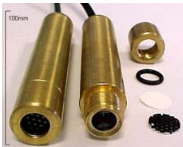
Fig. 1: Sensor design and exploded view of the head assembly. The sensor on the left is shown fully assembled. The sensor on the right shows an exploded view of the sensor head assembly.
