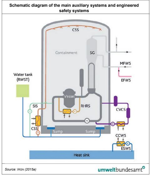
Figure 2: Schematic diagram of the main auxiliary systems and engineered safety systems.
