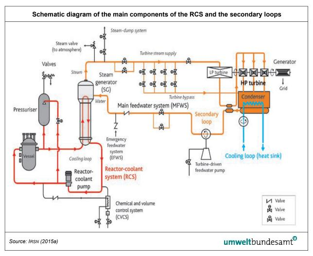
Figure 2: Schematic diagram of the main components of the RCS and the secondary loops.
