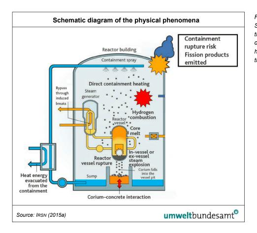
Figure 6: Schematic diagram of the physical phenomena occurring during direct heating of the gases in the containment.
