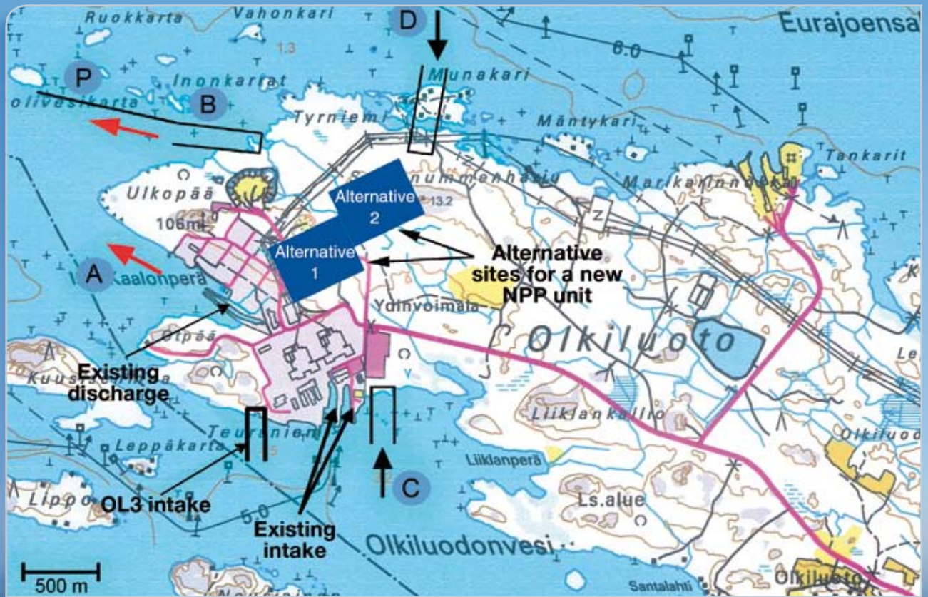
Figure 4-1 Alternative locations for the power plant unit and alternative locations for cooling water intake and discharge. A and B are locations for the cooling water discharge channel for plant unit 4, while C and D are locations for the cooling water intake channel for plant unit 4. P refers to a potential extension to the northern bank of discharge channel B in order to reduce the effect of water recirculation.
