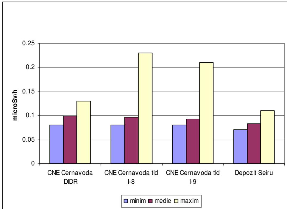
**Figure 4.2.1.4-5.** Gamma dose rates in air in the CNE – PROD Cernavoda site
