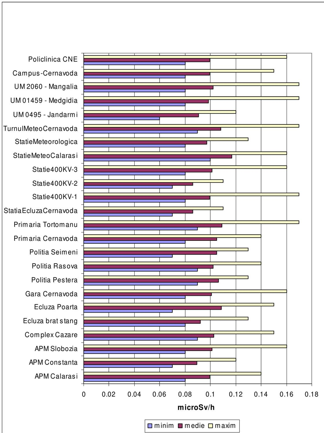
**Figure 4.2.1.4-6.** Gamma dose rates in air outside the CNE – PROD Cernavoda site
