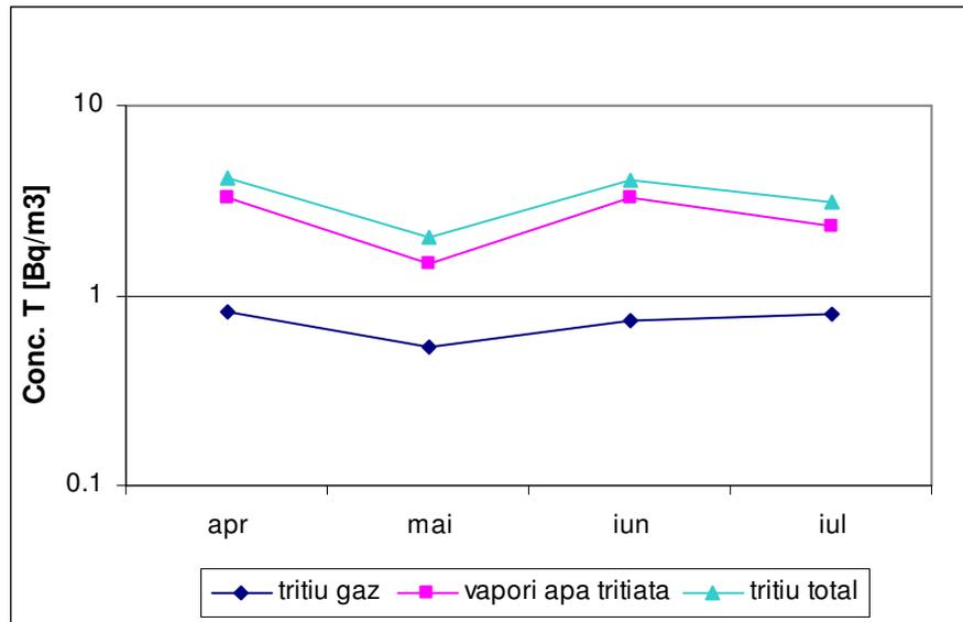
**Figure 4.2.1.4-3.** Concentrations of tritium gas, tritiated water vapors and total tritium in air - Campus Cernavoda - in the period April – July 2004
