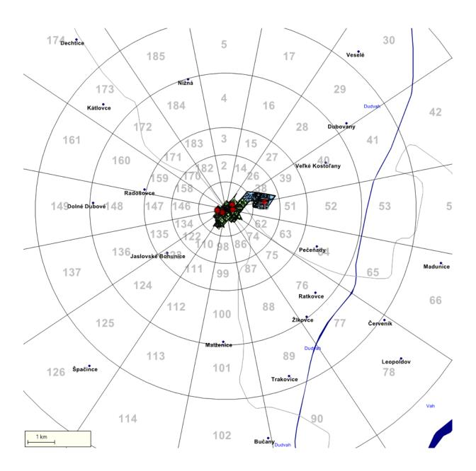
The plot of division of the area around the centre of the JAVYS, a.s. premises to sectors according to the ESTA AI programme for the calculation of impacts of released radioactive substances to a distance of  $100 \, \mathrm{km}$
