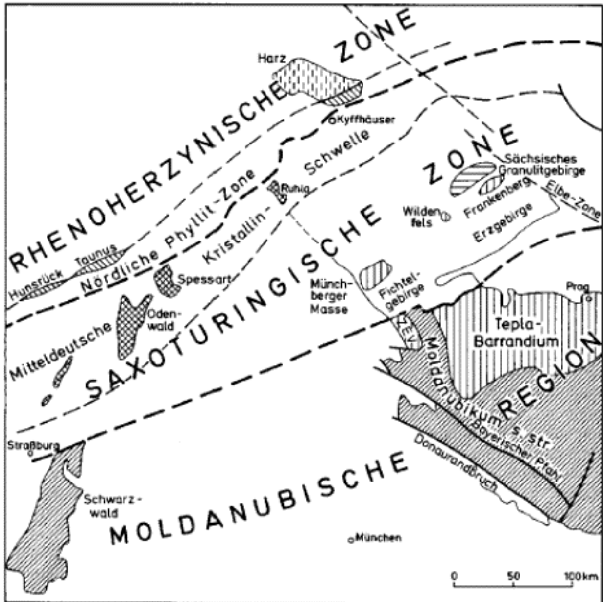
Figure 2.4.1: Geological overview: Major tectonic units of the Variscan Belt in Central Europe.
