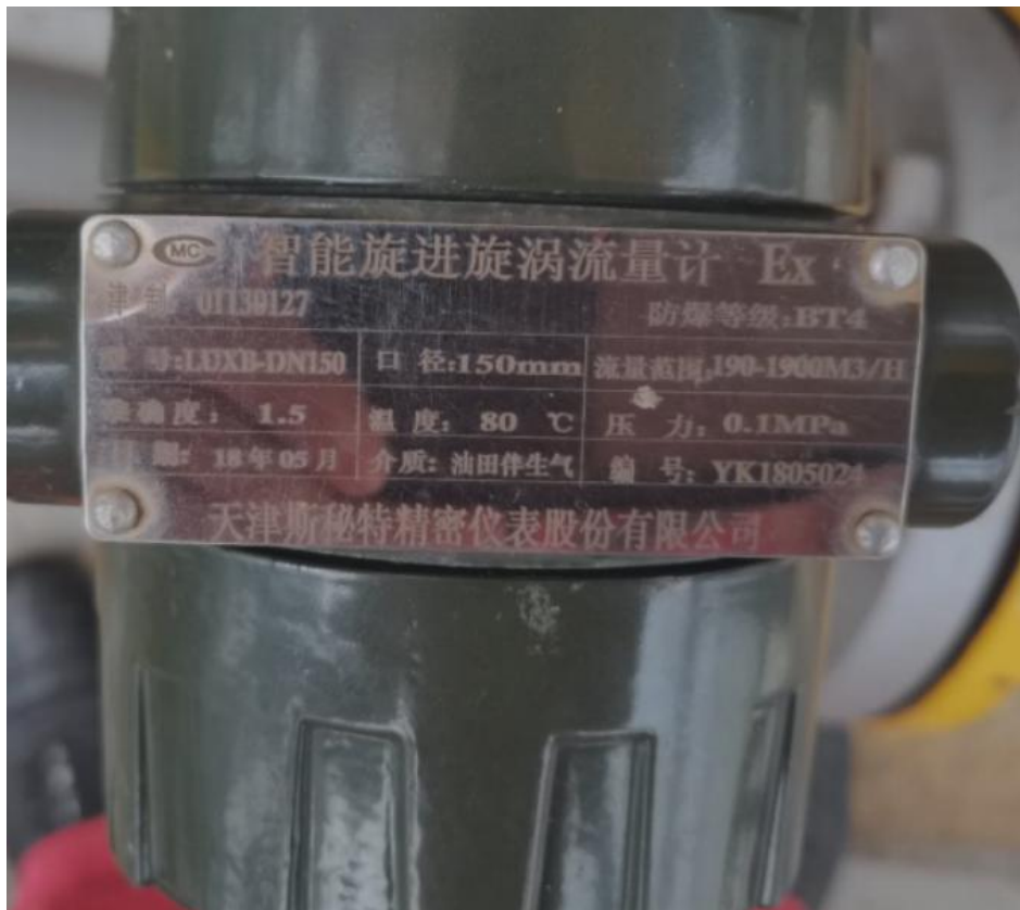
Image 3: Recovered gas flow-meter nameplate.
